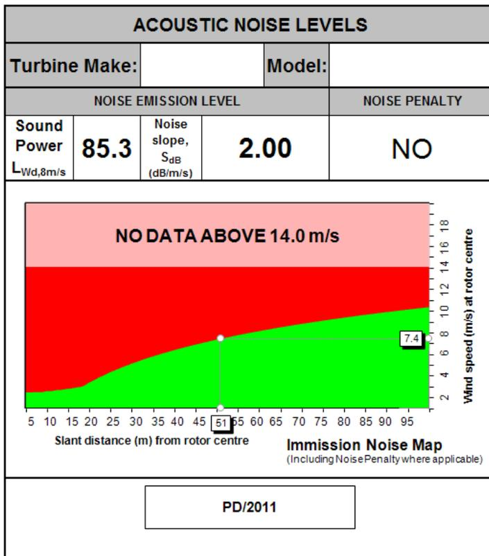
The noise map can be read by drawing a horizontal line from the recorded wind speed at hub (right hand side of the map) to where the red and green lines meet. Drawing a vertical line from
